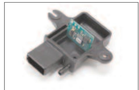
**Figure 2** A non-potted, partially assembled Airtex Engine Management MAP sensor, with board tilted to reveal ICs.
