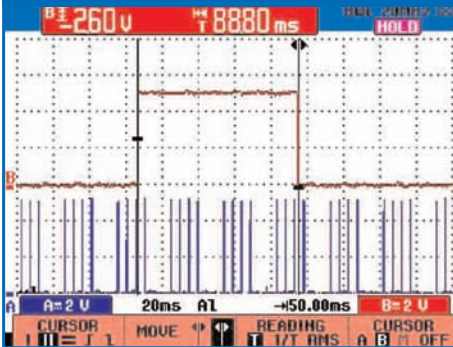
Figure 2: Bad cam and crank sensor SYNC waveforms.
