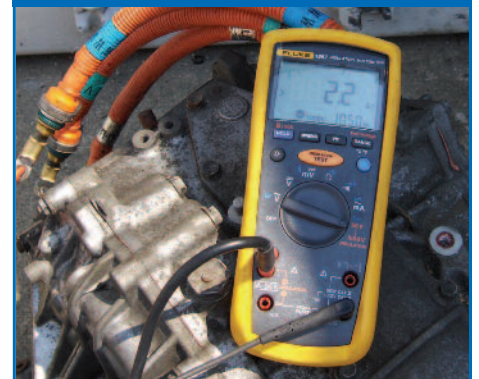
Figure 5: Second transaxle with good MG windings
