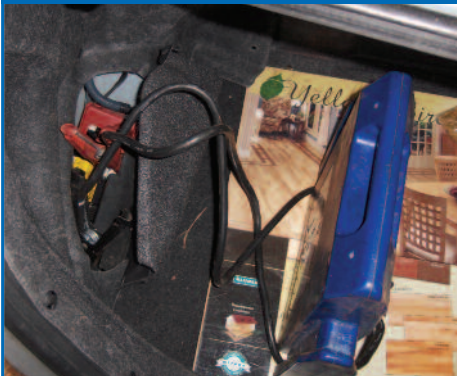
Figure 2: Installing battery pack on AGM battery
