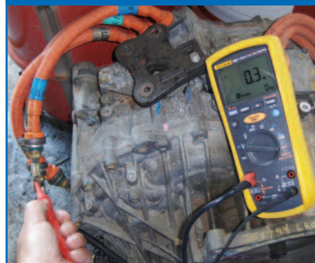
Figure 4: Hybrid transaxle with shorted MG windings
