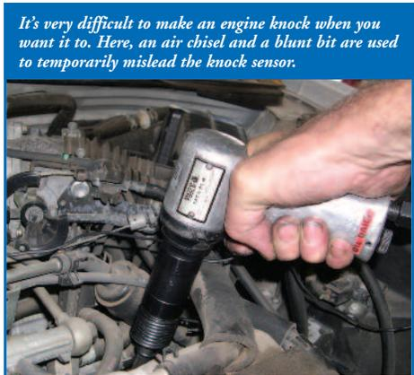
*It's very difficult to make an engine knock when you want it to. Here, an air chisel and a blunt bit are used to temporarily mislead the knock sensor.*
