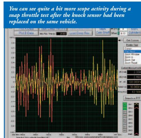
*You can see quite a bit more scope activity during a snap throttle test after the knock sensor had been replaced on the same vehicle.*
