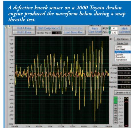
*A defective knock sensor on a 2000 Toyota Avalon engine produced the waveform below during a snap throttle test.*
