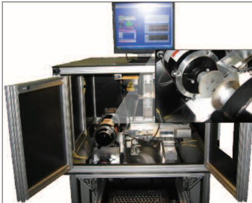
captured by a 14-bit analog device, then sent to the integral computer system (shown here) for analysis. Rejected sensors are scrapped and passing sensors are laser date coded.
