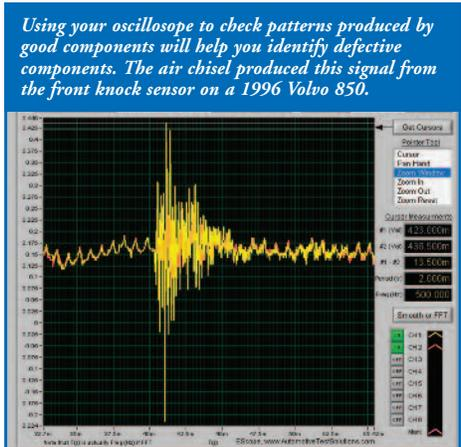
*Using your oscilloscope to check patterns produced by good components will help you identify defective components. The air chisel produced this signal from the front knock sensor on a 1996 Volvo 850.*
